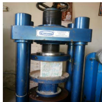
Fig. 4: Cube Test is in Progress for Compressive Strength
