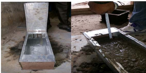
Fig. 2: L-Box test apparatus and Test reading
