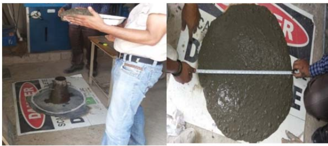
Fig. 1: Slump test apparatus and Test reading
